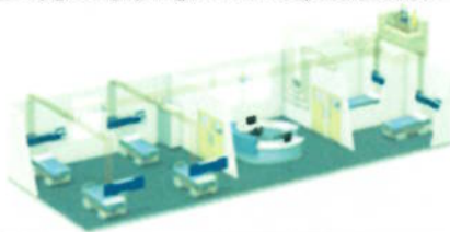
Oxygen piping in a hospital ward
